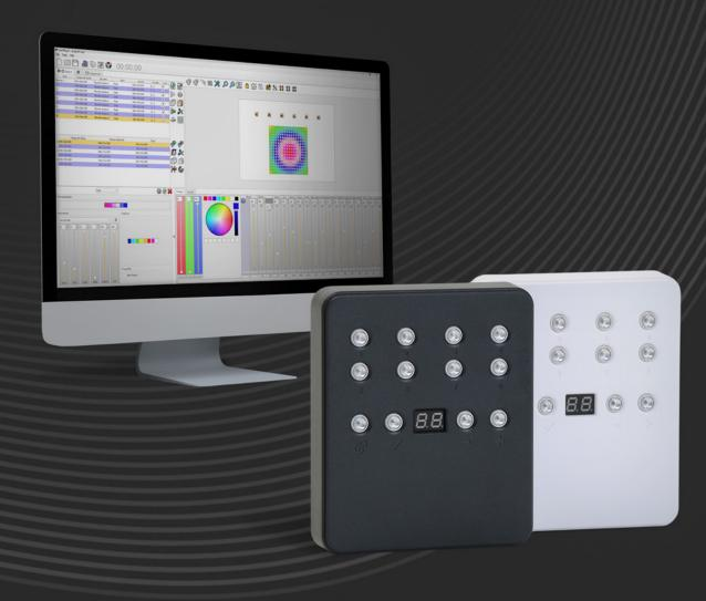
The SLIM Stand Alone interface provides a wall-mounted solution designed for indoor installations and projects requiring a user-friendly and aesthetically-pleasing lighting control panel.
